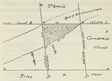
The triangle A, B, C, shows distance taken on the strike of the vein, and the surface of the Compromise Ground taken.
